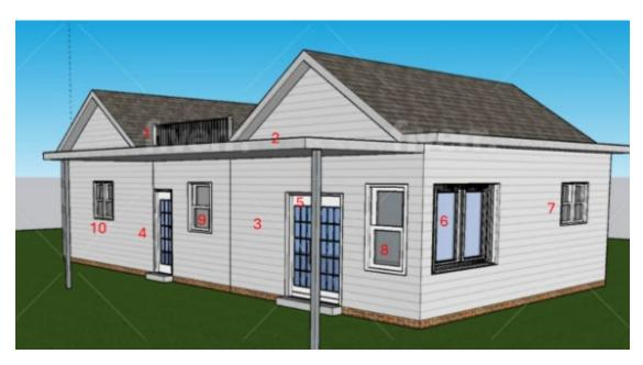
1. The rear flat roof line between the two peaks will be raised by 10". The slope will still start at the same point (below the upper level exterior rear door) and will slope more gently to meet the bottoms of the existing roof peaks. A black aluminum railing (216"w x 48"h) will be added to the end of the porch roof. (48x216)
